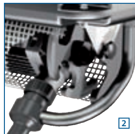
Drive Pump drive with venturi nozzle
